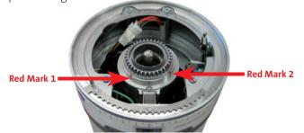
Therefore turn the grind adjustment of the built-in grinder to the right red mark 2 for refitting the grinder's lid.
